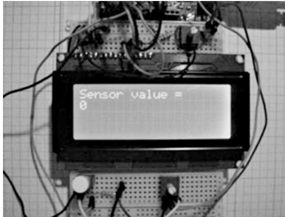
Figure 8-27. Low-cost proto-evaluation breadboard. The push-button switch and potentiometer allow quick evaluation of the Manual Counter and Read Sensor sketches.
