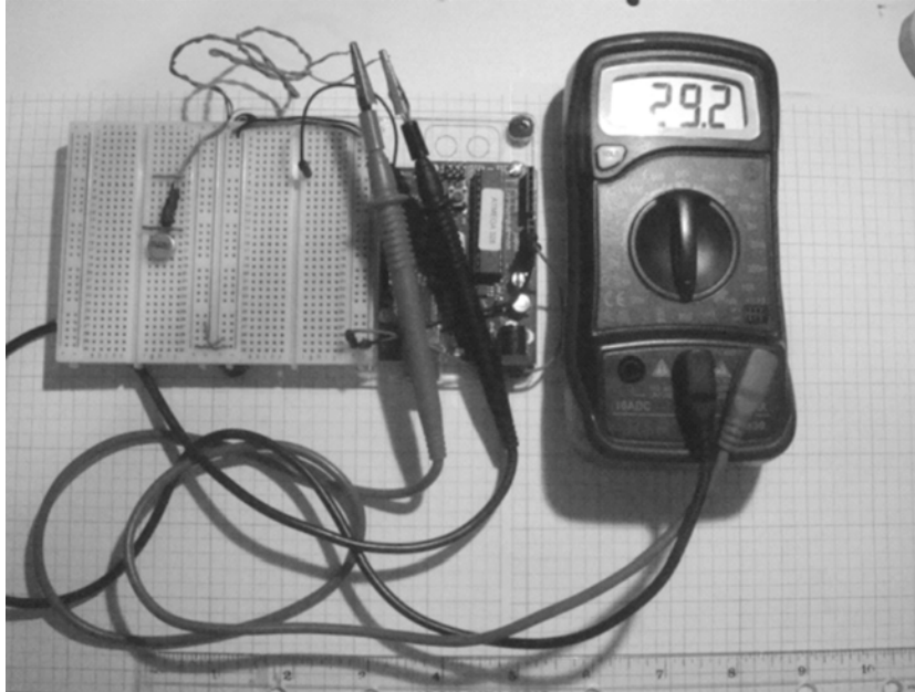
Figure 7-8. Measuring the vibration motor's R_a using a DMM (digital multimeter) ohmmeter
