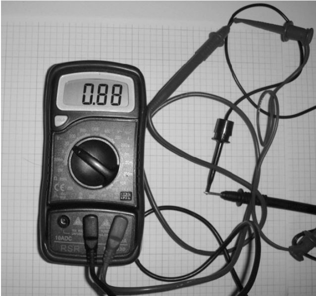
Figure 1-21. Ambient light based on the DMM's LCD voltage drop reading of the photocell
