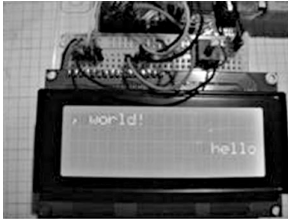
Figure 8-20. The “hello, world!” message scrolling left and right on the LCD
