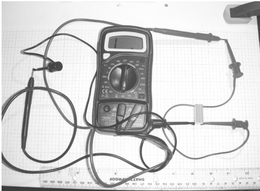
Figure 2-10. A typical setup for testing a LED bar display using a DMM
