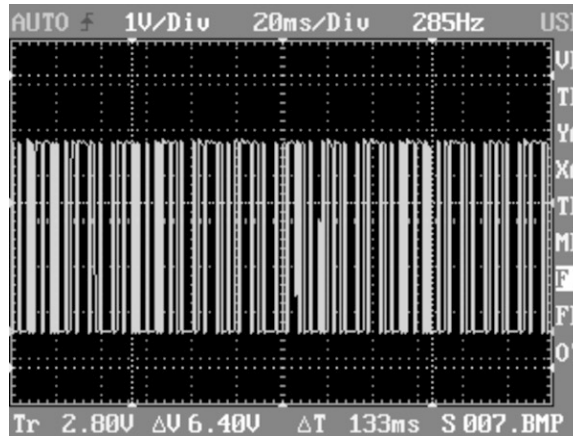
Figure 7-21. A 285 Hz PWM signal based on a 1200 stepsPerRevolution value
