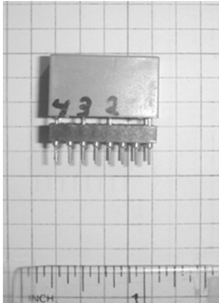
Figure 4-13. An IC socket used to improve the insertion of the electromechanical relay onto the solderless breadboard
