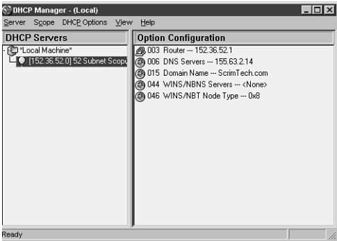
FIGURE 4.9 The DHCP Manager with options set. Options with an icon of a group of computers are scope options; the icon globes refer to global options.
