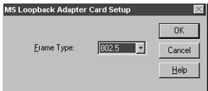
FIGURE 2.3 The Setup dialog box for the MS Loopback Adapter.
