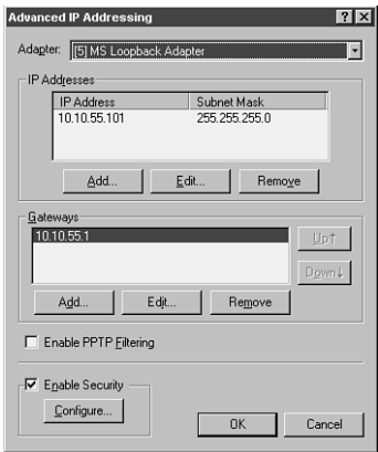
FIGURE 2.13 You can add extra IP addresses and gateways and perform other configurations in the Advanced IP Addressing dialog box.
