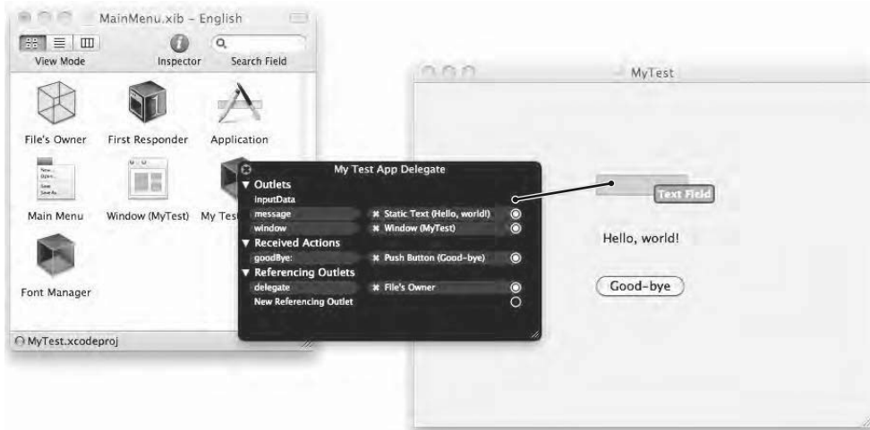
Figure 3–10. Dragging from the inputData circle to the text field connects the text field to the inputData Outlet defined in your Objective-C code.
