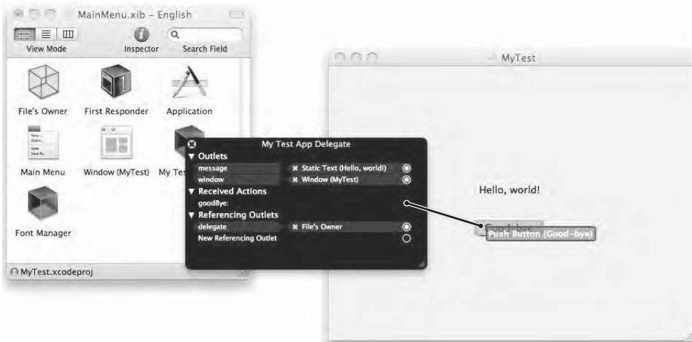
Figure 3–9. Dragging from the Actions circle to the user interface connects the Action method to the push button object.
