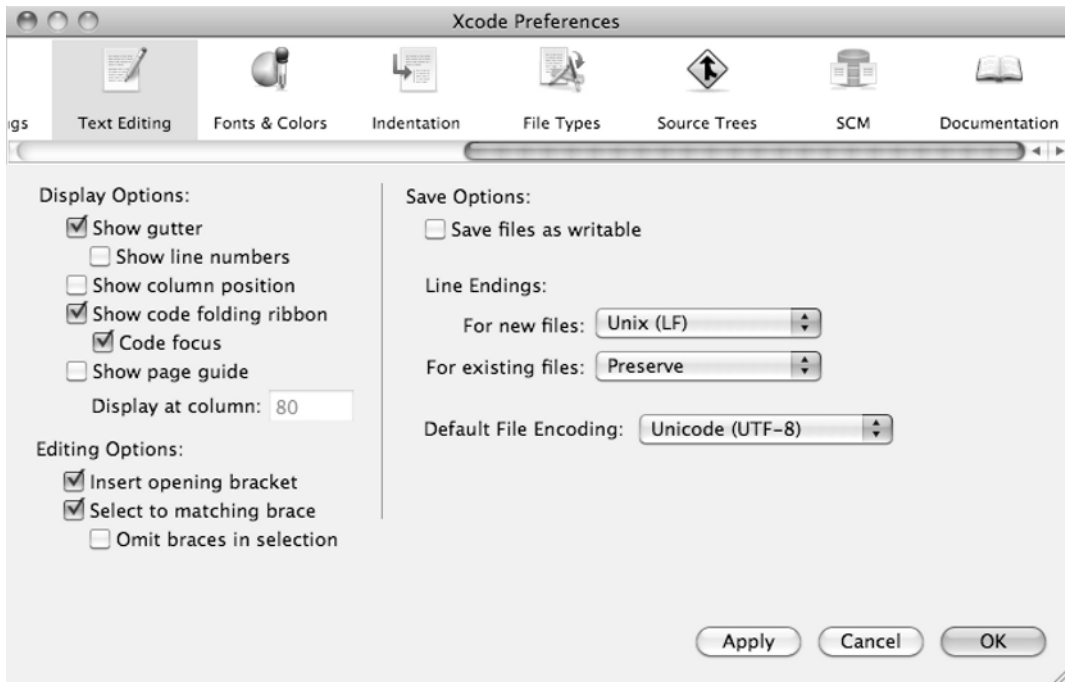
Figure 4–13. The Text Editing icon displays ways to modify the appearance of Objective-C code in the editor.
