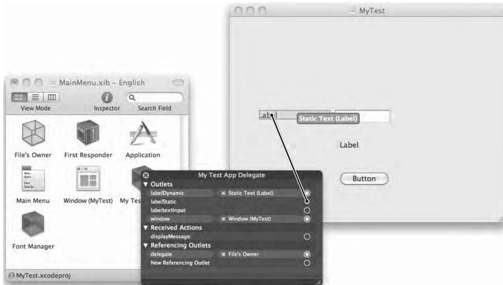
Figure 18-4. Dragging and dropping connects the labelStatic IBOutlet to your label on the user interface.
