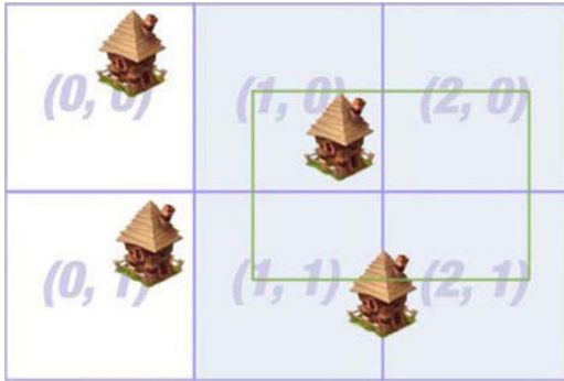
Figure 7-16. An example of cluster layout. The viewport intersects four clusters. Only two objects participate in rendering.
