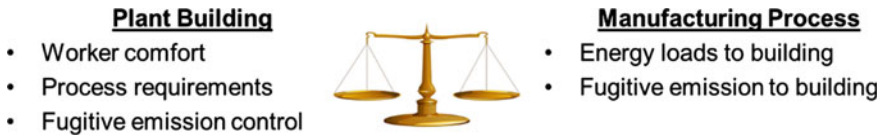
Fig. 7.1 Plant building and manufacturing process energy balance
