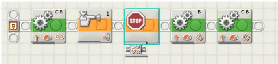
Figure 13-17. Use of the Stop block
