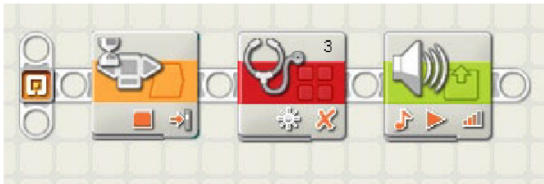
Figure 8-7. A program to delete the current Light sensor calibration
