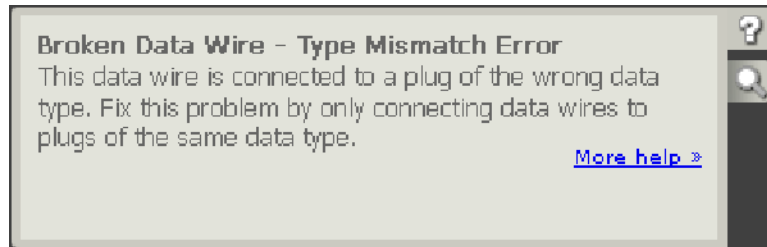
Figure 5-3. A broken data-wire message in the Help panel
