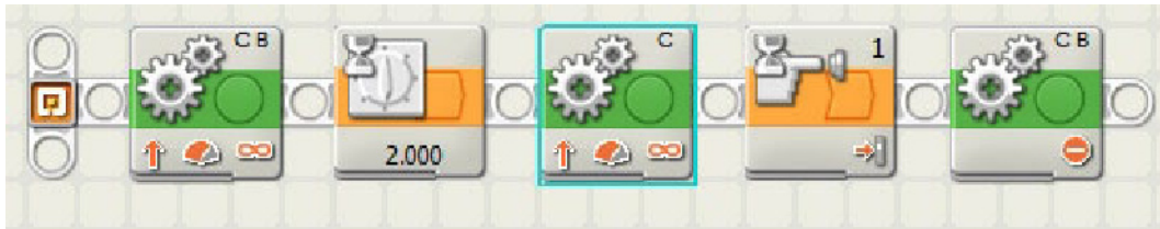
Figure 14-7. Drive, then turn example (error)
