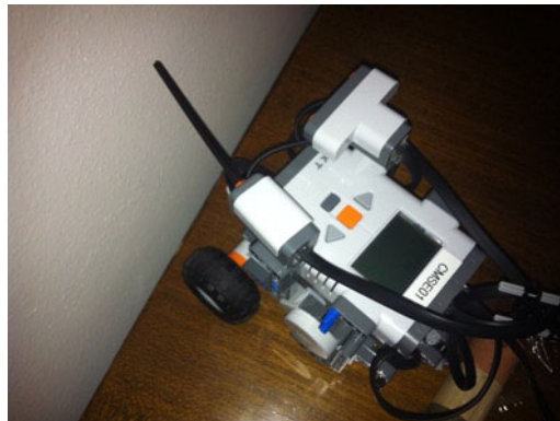
Figure 9-5. The Touch sensor is too close to the obstacle
