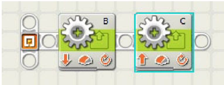
Figure 7-10. Motor blocks on the same sequence beam
