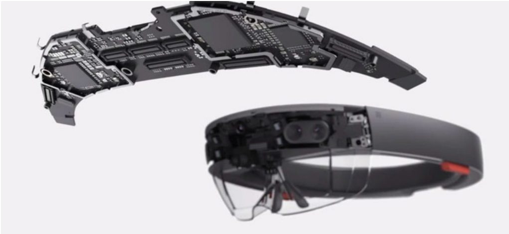
Figure 13-2. The HoloLens processors on the main logic board
