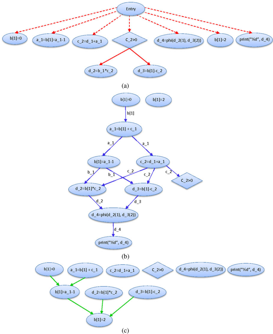
Fig. 2.14 Control dependence graph (a), data dependence graph (b), anti-dependence graph (c)
