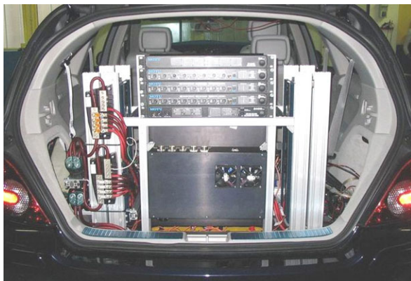
Fig. 5.9 PowerServer final setup in the car trunk
