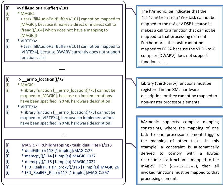
Fig. 4.15 A description of some of the hArtes constraints automatically derived by the hArmonic tool to ensure that the mapping solutions are feasible on the hArtes platform. This figure shows part of the log generated by hArmonic when processing the beamformer application. A total of 677 mapping constraints are identified for this application
