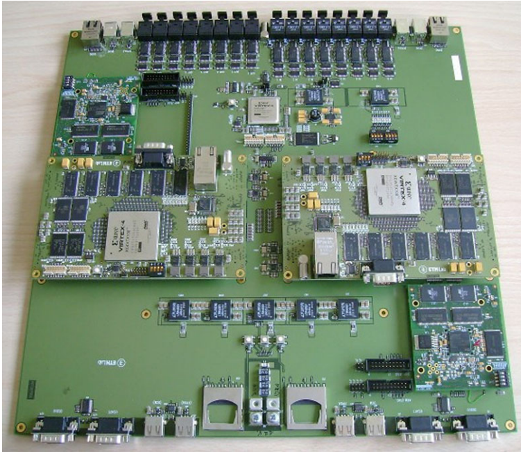
Fig. 3.5 Picture of the hArtes Hardware Platform. The two BCEs use two daughter boards each, one for the D940HF processor and one for the FPGA based infrastructure. These daughter-boards are at the center of the mother board. The ADAT interfaces and several standard I/O connectors are clearly visible at the top and at the bottom of the picture, respectively
