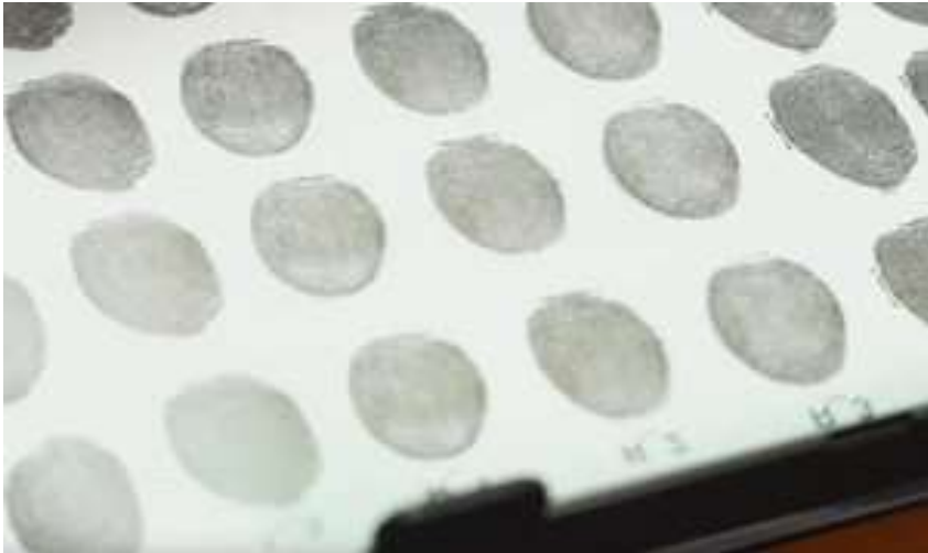
Figure 1. Fingerprints printed using a standard inkjet printer loaded with capacitive ink and insulating paper can trick smartphone fingerprint sensors. (Photograph: Michigan State University)
