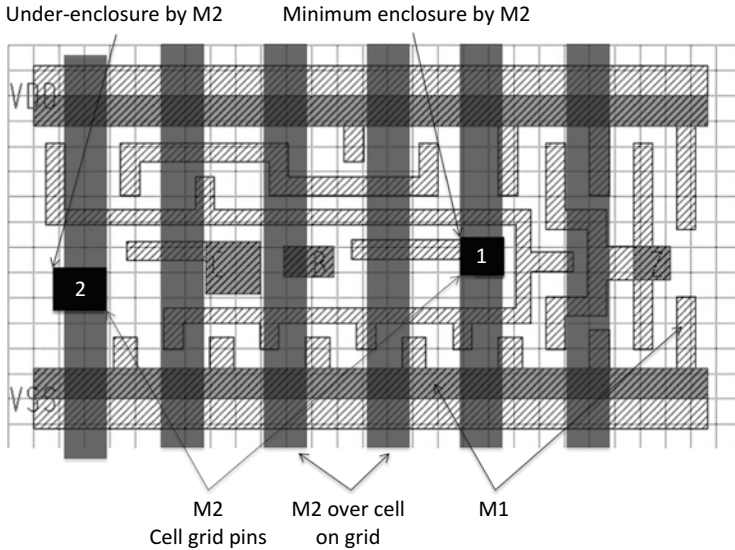
Fig. 3.17 Cell pin rectangles on Metal1 (1 and 2) must fully enclose Metal2 routing aligned to the Metal2 grid. Property values on error marker should help designers to determine how much positive or negative enclosure exists, so designers can determine how best to fix the violation (after [9])
