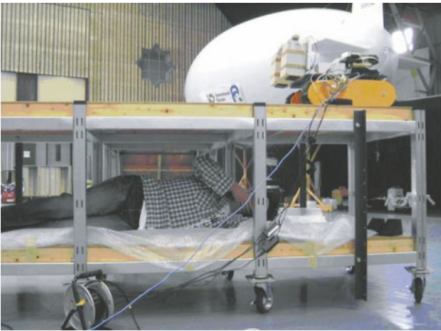
Fig. 6.16 Radar system on the HELIOS Carrier is moved to transmit UWB pulses down toward a subject
