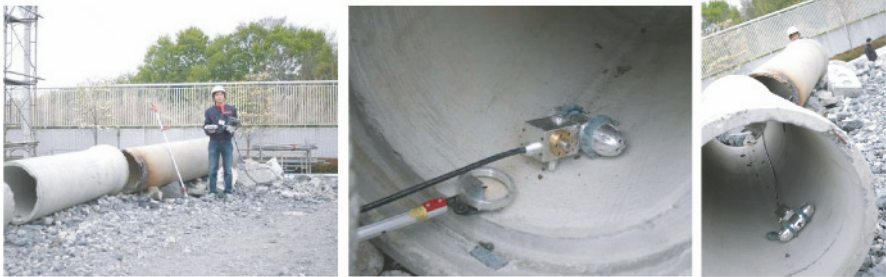
Fig. 5.29 Practical application verification experiment: running through disconnected cylinders
