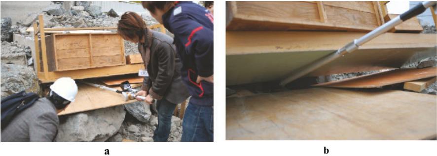
Fig. 5.27 Using the Strong Search Cam. a Pushing into narrow space. b Using like crowbar
