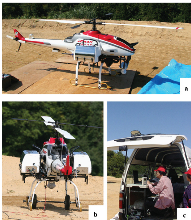
Fig. 3.5 Intelligent aerorobot developed by Kyoto University group: a intelligent aerorobot's side view. b Rear view. c Van for robot transportation, equipped with control and monitoring devices
