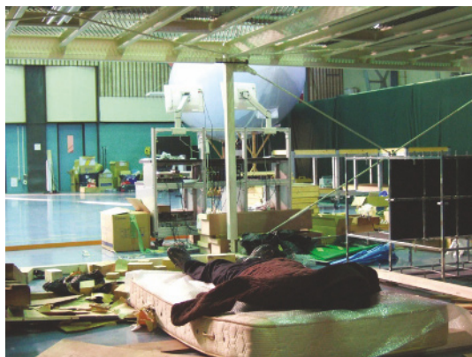
Fig. 6.18 Feasibility experiments of the radar system on the HELIOS Carrier. a Radar system on the Helios carrier moves on a wooden board on the second floor of the test field. b Subject lying on the first floor of the test field
