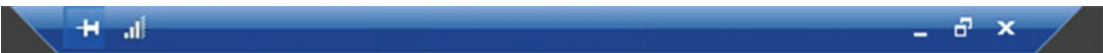
Figure 12-35. Full-screen Remote Desktop is controlled by a bar at the top center of your screen
