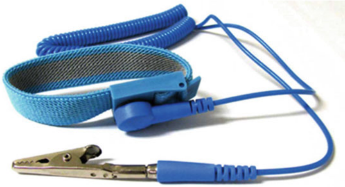
Figure 29-2. An antistatic wristband can protect delicate electronics
