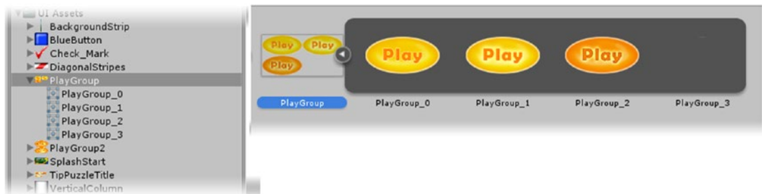
Figure 10-21. The sprites generated from the atlased texture sheet, One Column Layout (left), and Two Column Layout (right)
