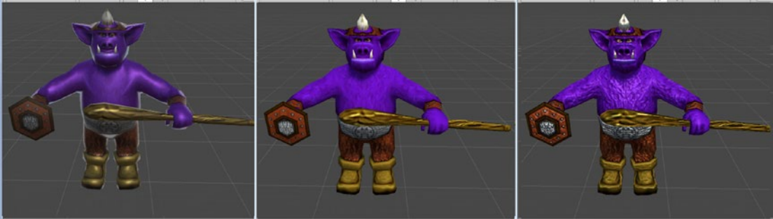
Figure 4-54. The default Diffuse shader (left), the Specular Bump shader before adding the normal map (center), and after adding the normal map (right)
