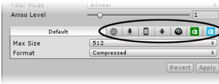
Figure 4-33. Override choices: for Web, stand-alone (desktop), iPhone, Android, BlackBerry, Windows Store apps, and Windows Phone 8
