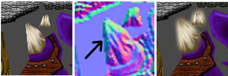
Figure 4-55. The horn in the original texture (left), the normal map it generates (center), and a method of reducing seams created when the surrounding color contrasts too much (right)
