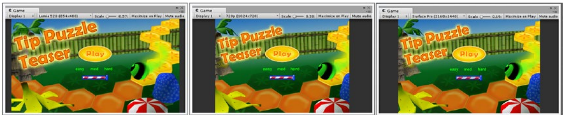
Figure 10-31. Slight scaling of the Title image between the Lumia (left), 720p (center), and Surface Pro (right) screen presets
