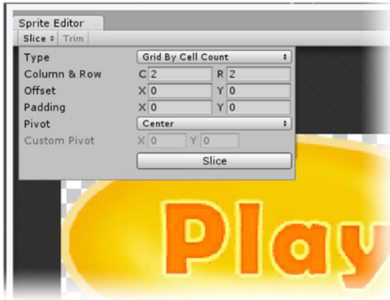
Figure 10-20. Using the Grid By Cell Count option to separate the atlased texture sheet
