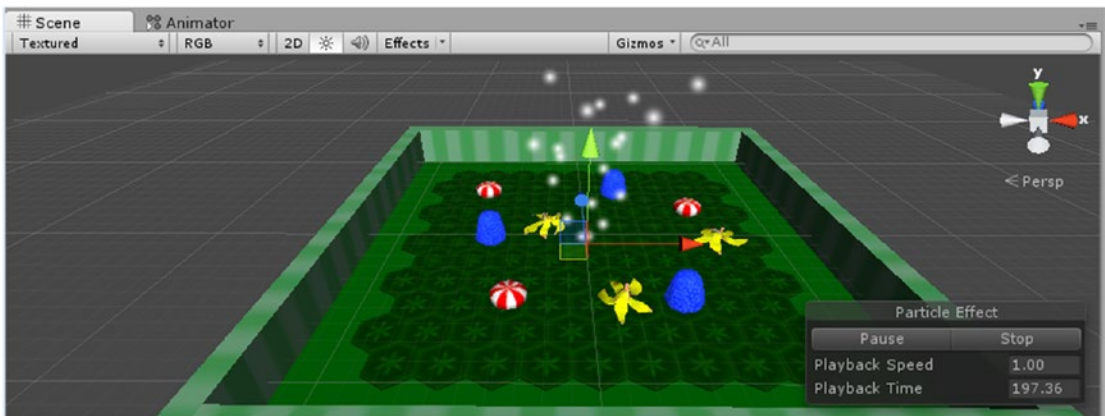
Figure 9-8. The selected Shuriken particle system and its Particle Effect dialog box in the Scene view
