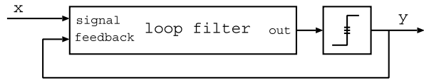
Fig. 5.1 Generic model of the Sigma-Delta noise-shaping loop, consisting of 2-input loop filter and quantizer
