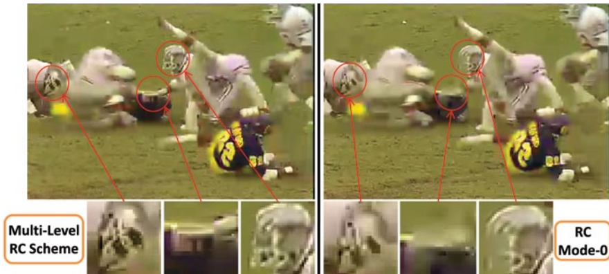
Fig. A.10 Evaluating the image and motion based MB prioritizations (Note: All excerpts are 2× zoomed using nearest neighbor interpolation)
