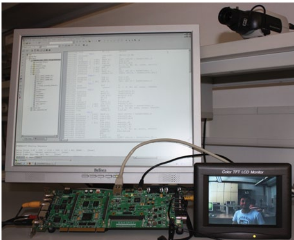
Fig. B.4 H.264 video encoder executing on the TI' DM6437 DSP board
