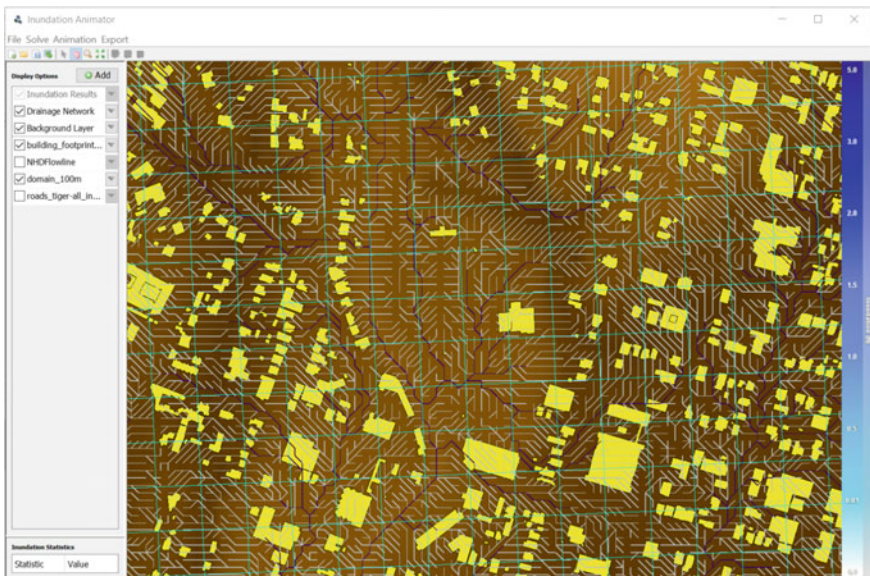
Fig. 12.11 Processing a high-resolution flow direction for use inundation analyst
