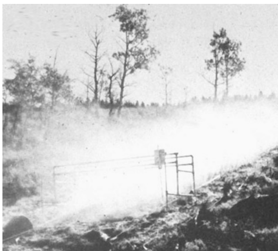
Fig. 6.2 Rainfall simulator for measuring hydraulic roughness at Boulder Creek Site 2. Emmett (1970)
