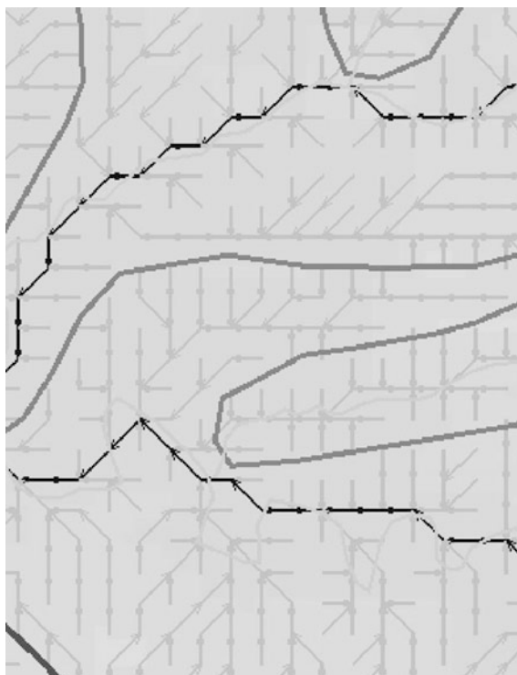
Fig. 7.10 Constrained drainage direction map with the delineated stream shown in black
