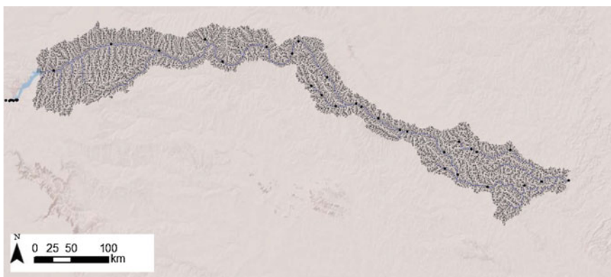
Fig. 11.14 Lower Canadian River model with sampling sites ( black circle icons ) superposed on the drainage network with overland cells ( gray ) and channel cells ( blue )
