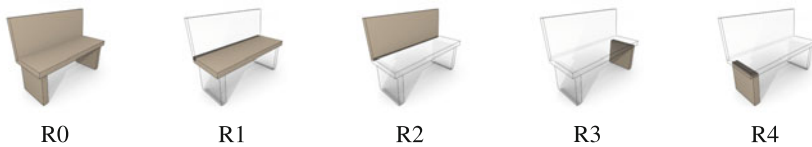
Fig. 12 Ontology and meshes used for our experiments on furniture segmentation and annotation. Right result of the segmentation and annotation on 5 objects from the furniture domain. Result of the annotation: orange \Rightarrow backrest, blue \Rightarrow seat, other colors \Rightarrow feet
