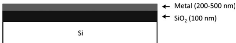
Fig. 7.3 Cross-sectional view of deposited metallic films on \text{SiO}_2 -Si substrates
