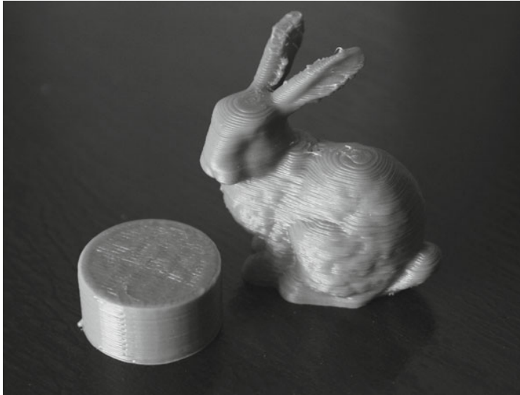
Figure 3-11. Example of solid layers
