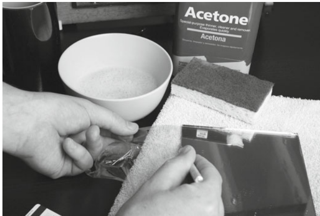
Figure A-7. Trimming polycarbonate tape with a hobby knife
