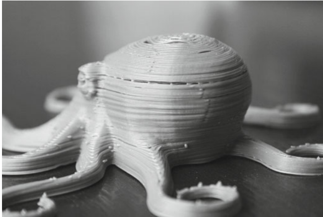
Figure A-12. Thin layers during a print
