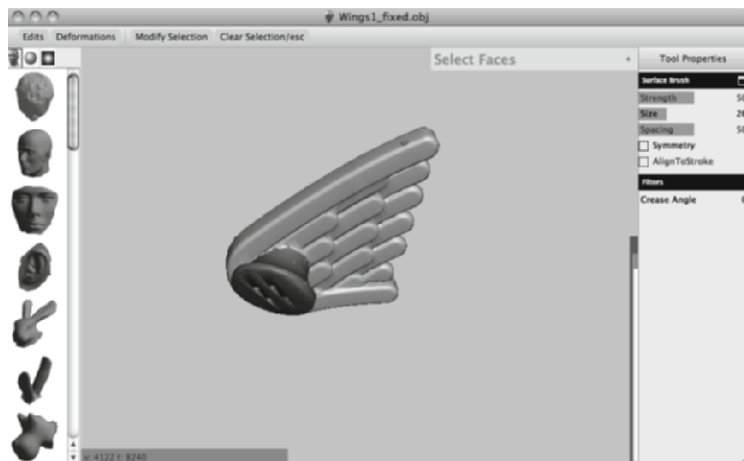
Figure 7-21. Removing stand from wing
