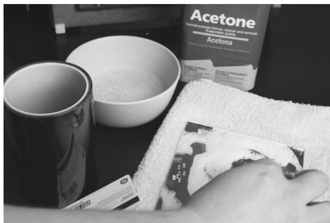
Figure A-4. Wetting the surface with soapy water
