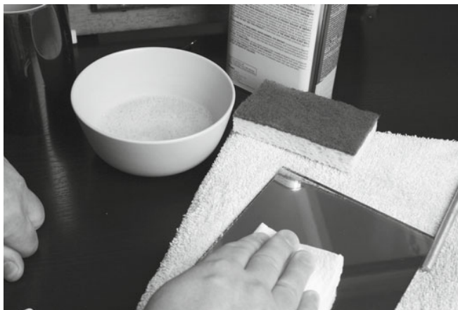
Figure A-8. Cleaning new tape with acetone
