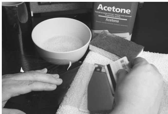
Figure A-6. Removing soap and water from underneath the tape
