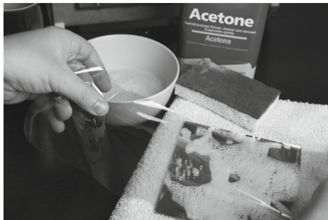
Figure A-5. Applying polymide tape to soapy surface
