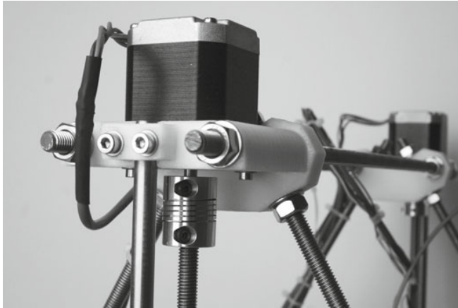
Figure 10-8. Aluminum helical coupler on a RepRap z-axis
