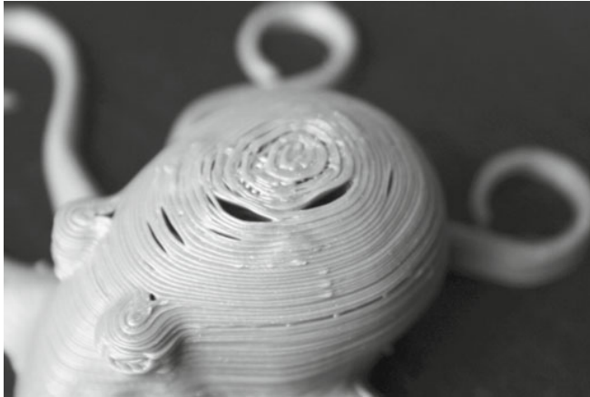
Figure A-13. Gaps in a print
