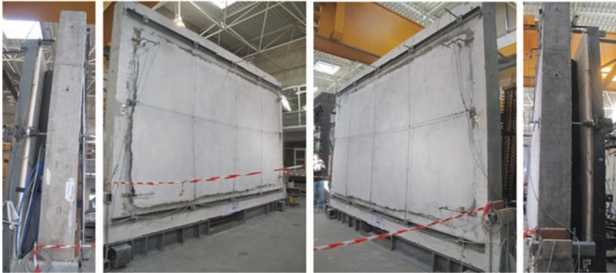
Fig. 12.19 Test 2, point 5. Deformation of the infill at \sim 50 mm of displacement of control point 8
