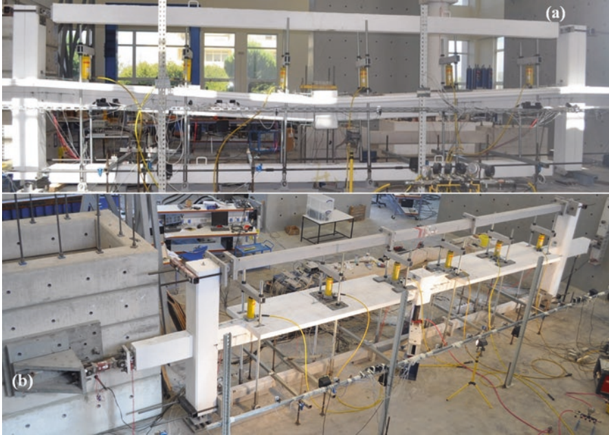
Fig. 2.15 Frame subassemblies after test: (a) monolithic; (b) precast, with dry-joints and concentric pre-stressing of the beam
