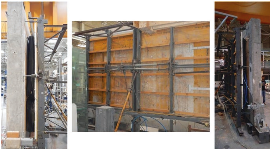
Fig. 12.6 The airbags used to apply the load; left and right : lateral views; center : rear view
