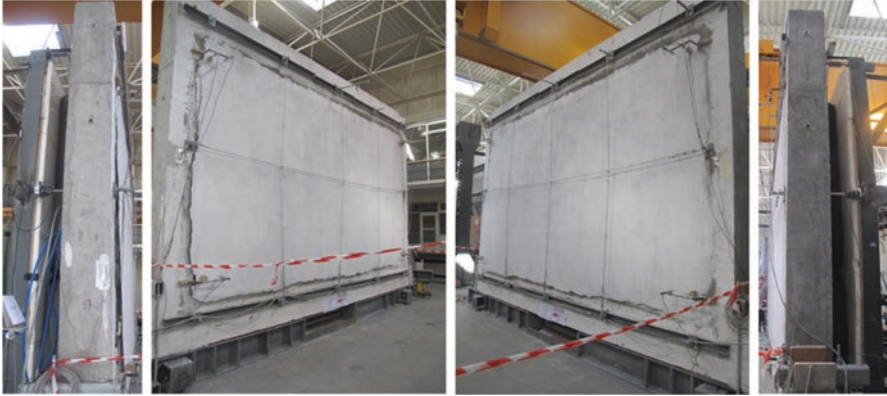
Fig. 12.18 Test 2, point 4. Deformation of the infill at \sim 40 mm of displacement of control point 8
