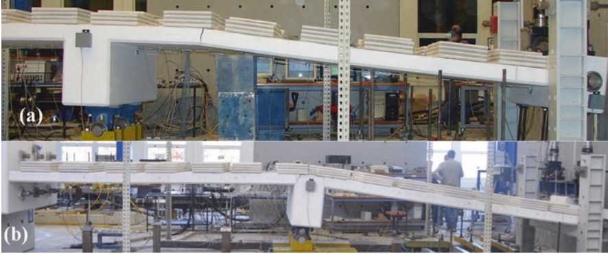
Fig. 2.14 Slab tests and failure mode: (a) discontinuous top reinforcement; (b) continuous top reinforcement
