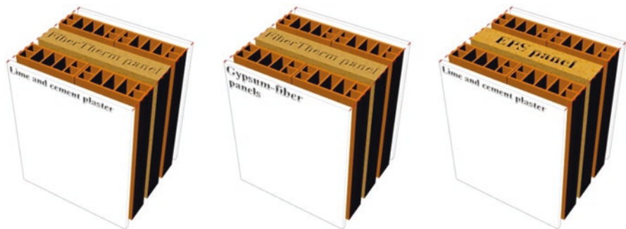
Fig. 12.26 Section view of the different proposed stratigraphies
