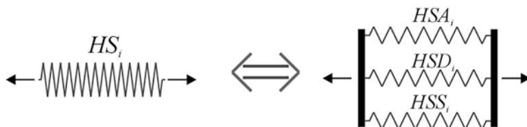
Fig. 5.6 Each horizontal spring is composed of 3 components to account for aggregate interlock ( HSA ), dowel ( HSD ), and shear/horizontal reinforcement ( HSS ) mechanisms
