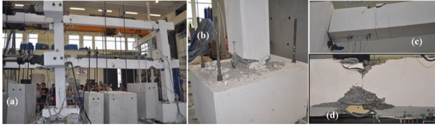
Fig. 2.5 Fixed-base dry-jointed frame: (a) maximum overall deformation; (b) typical damage, column base; (c) opening of dry joint at column face and of interface of precast segment with cast-in-situ concrete at top story beam; (d) typical damage around interface of precast and cast-in-situ parts of ground story beam
