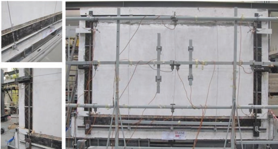
Fig. 12.9 Third test specimen with surface finish made by plaster and retaining plastic mesh. The smaller pictures show the connection system along the edges
