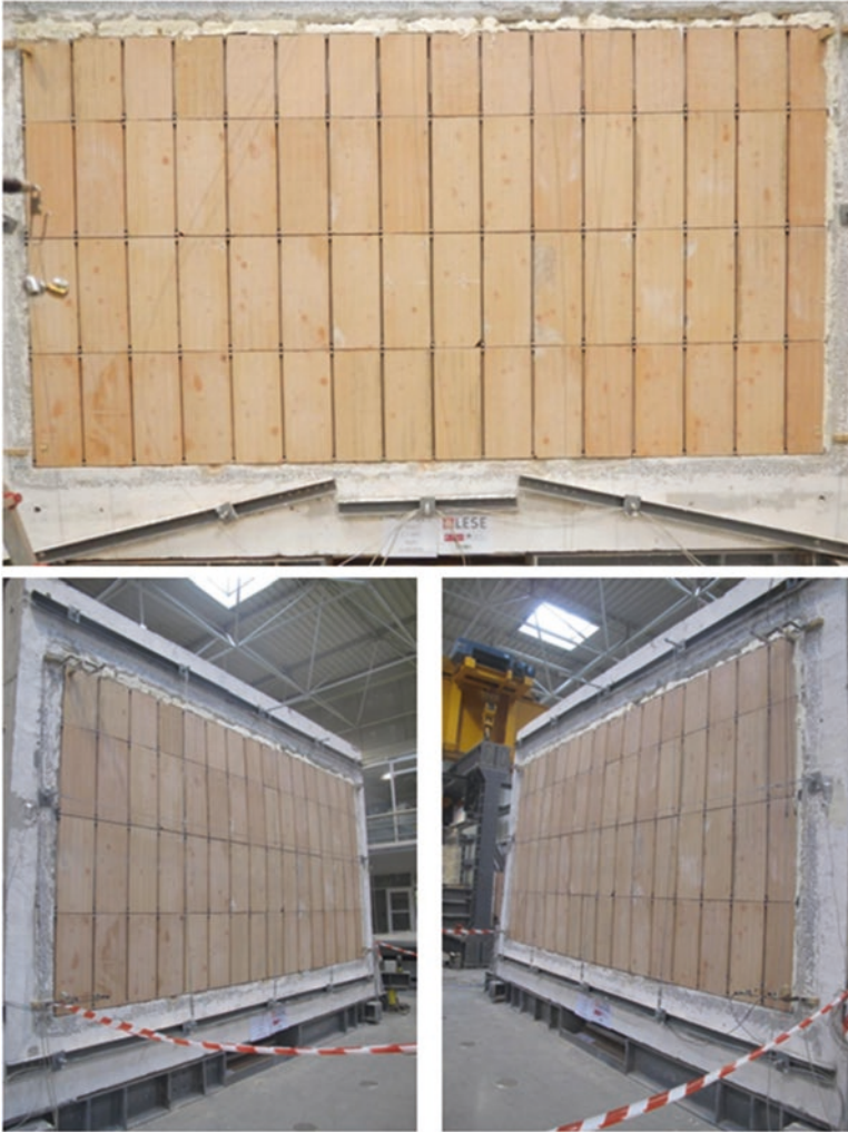
Fig. 12.13 Test 1, point 3. Residual deformation of the infill at zero pressure in the airbags
