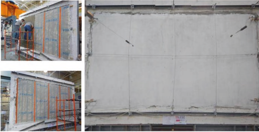
Fig. 12.8 Second test specimen with surface finish made by plaster and retaining plastic mesh
